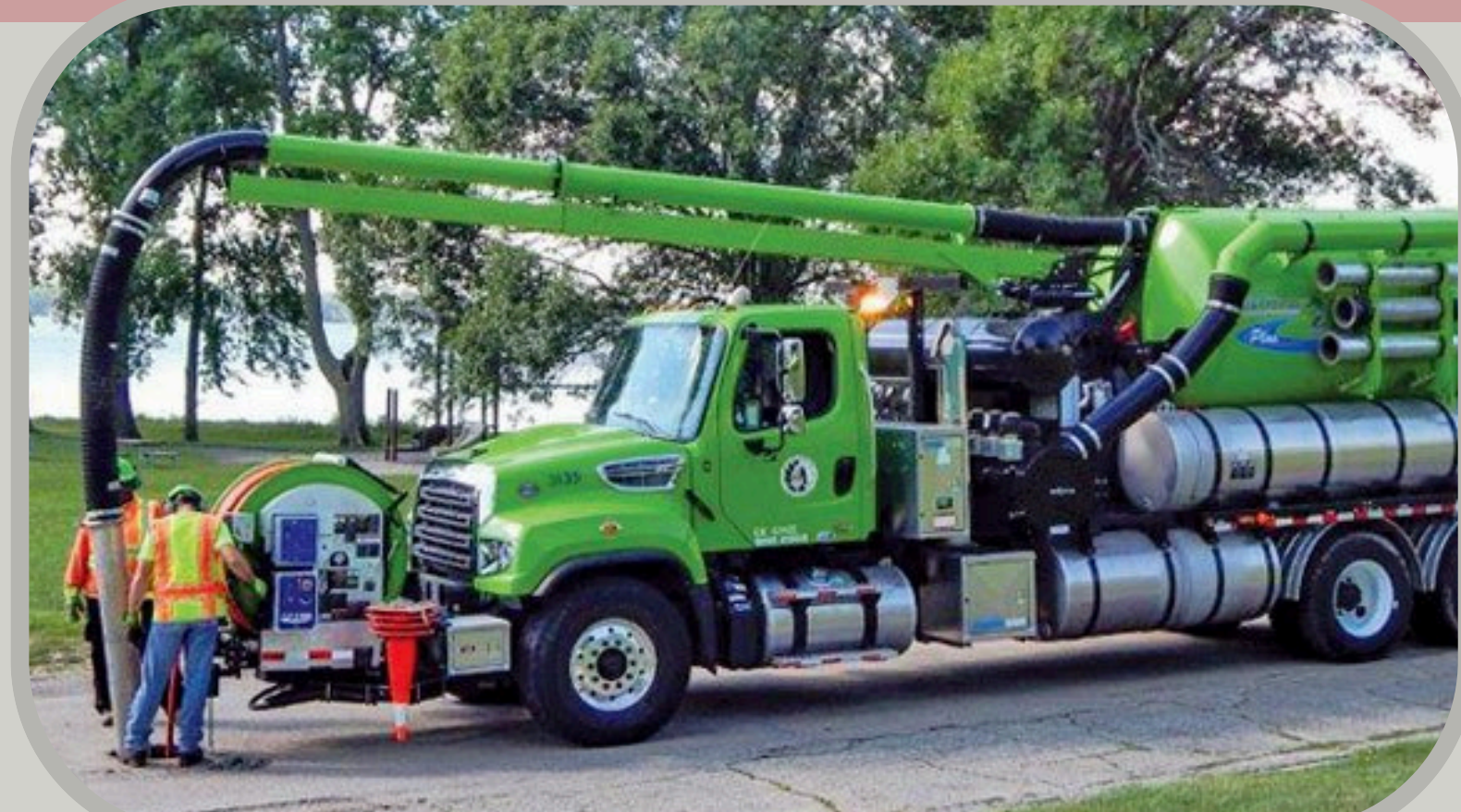
Vactor Truck used to clean sewer and address emergency back-ups
